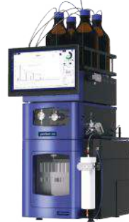
puriFlash® 5.050 250 mL/min - 50 bar Cross-over Flash /Prep
