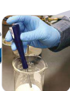
ASAP®: Atmospheric Solids Analysis Probe
