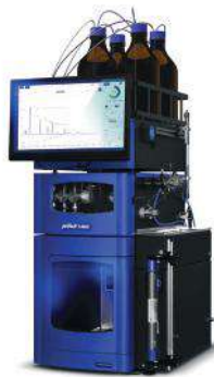
puriFlash® 5.400-UV 125 mL/min - 400 bar The Ultra-Purification
