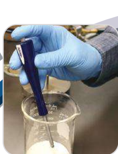
ASAP ® : Atmospheric Solids Analysis Probe
