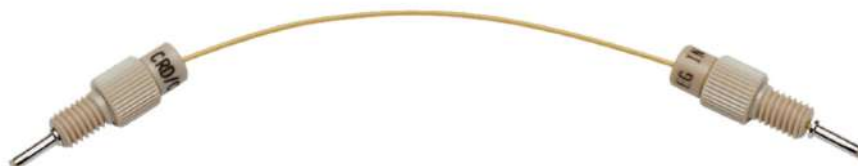
Figure 7. For best chromatographic performance, Dionex IC PEEK Viper fittings and sample loops are recommended for use with Dionex IonPac AS32-Fast-4 \mu m columns.
