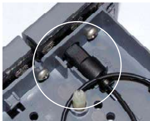
Figure 5 Column Outlet Fitting Installed in Column Cartridge
