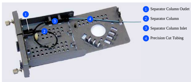
Figure 14 Separator Column Only Installed in Column Cartridge
