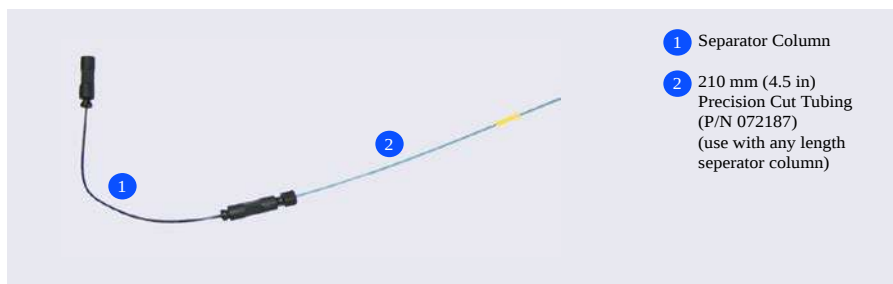
Figure 16 Tubing Connections for Separator Column Only
