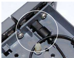
Figure 17 Column Outlet Fitting Installed in Column Cartridge
