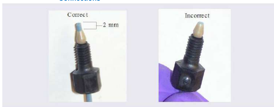
Figure 20 Correct and Incorrect Ferrule and Fitting Bolt Placement for Capillary Tubing Connections
