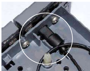
Figure 5 Column Outlet Fitting Installed in Column Cartridge
