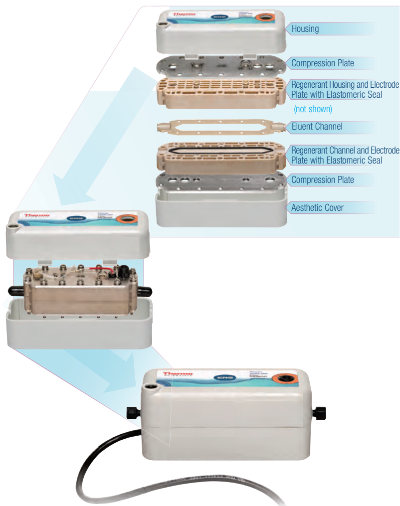
Figure 2. The Dionex ERS 500 suppressor components and assembly
