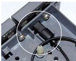
Figure 5 Column Outlet Fitting Installed in Column Cartridge
