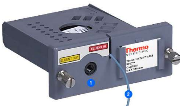
Figure 6. Column Cartridge Closed
