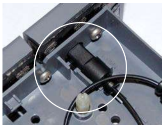
Figure 5. Column Outlet Fitting Installed in Column Cartridge
