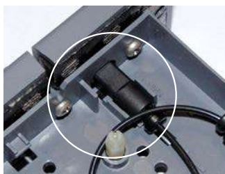
Figure 5 Column Outlet Fitting Installed in Column Cartridge
